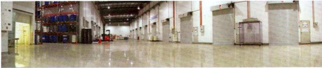
**Figure 1 : 9 separated room specially design for segregation of incompatible chemical Example Flammable, Toxic, Oxidising & Corrosive.**
